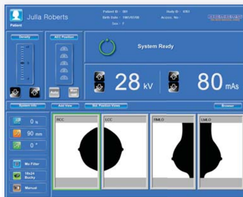
Synchronizing operation and display all parameters at PC and Main OP
